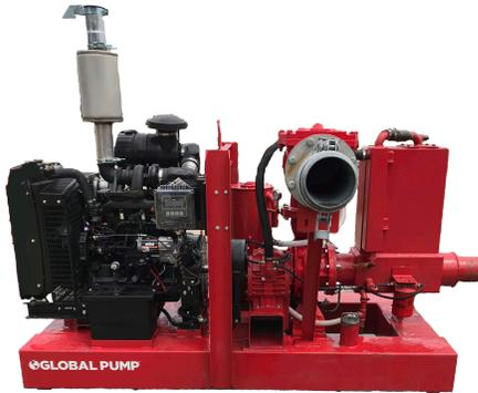
Global Pump® Standard Centrifugal Wellpoint pumps are specifically designed to effectively handle the arduous requirements of wellpoint and underdrain dewatering systems where intermittent water flow and large amounts of air are encountered. The dual diaphragm priming system generates up to 100CFM without the need for an oil-cooled vacuum pump.
